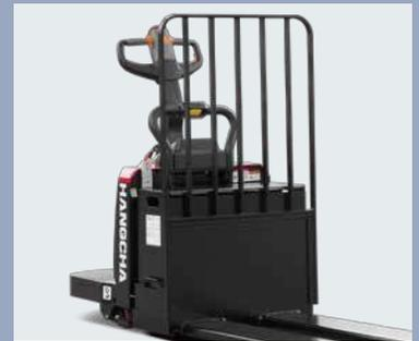
The load backrest is secured with high-strength bolts, which can protect the operator effectively
